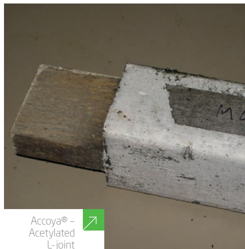
Accoya® - 42 months external coatings test
