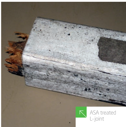
Pine - 42 months external coatings test
